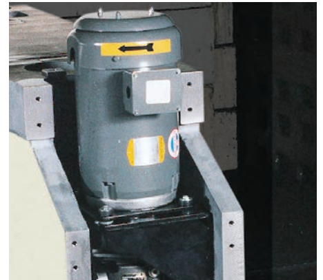
Hydraulic motor pump assembly mounted in left hand rear press bed leg.
