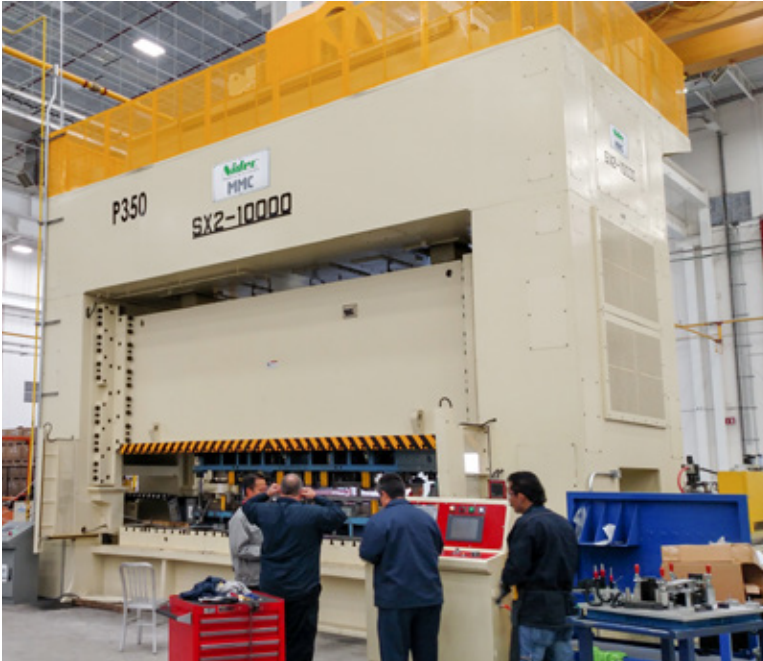
1,000 Ton Automotive Seating Structure Stamping Line in Mexico
