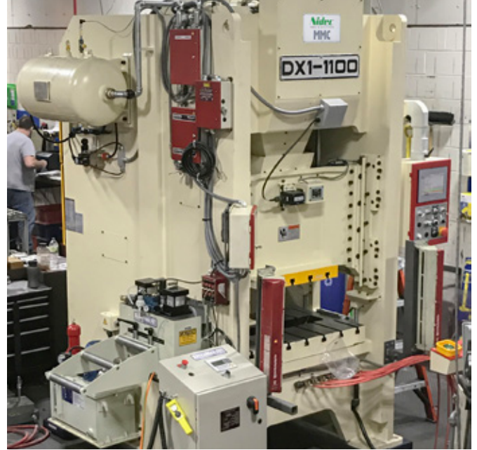
110 Ton D-Frame Press with Wintriss Automation Control for Tier 1 Appliance Customer in USA
